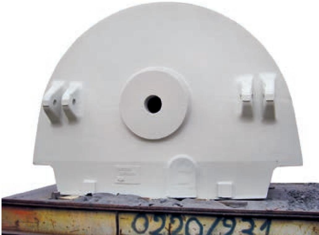
Cast component for a tile press
