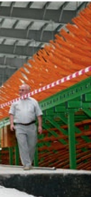
The Ecoformer SL had its premiere. For the first time, this system is integrated in a production plant at Uvadrev. This innovative surface layer wind former provides for homogeneous distribution of the surface layer particles while, at the same time, reducing material and energy consumption. The absolutely smooth surface now makes the use of especially light papers with delicate colors and intricate designs possible.
