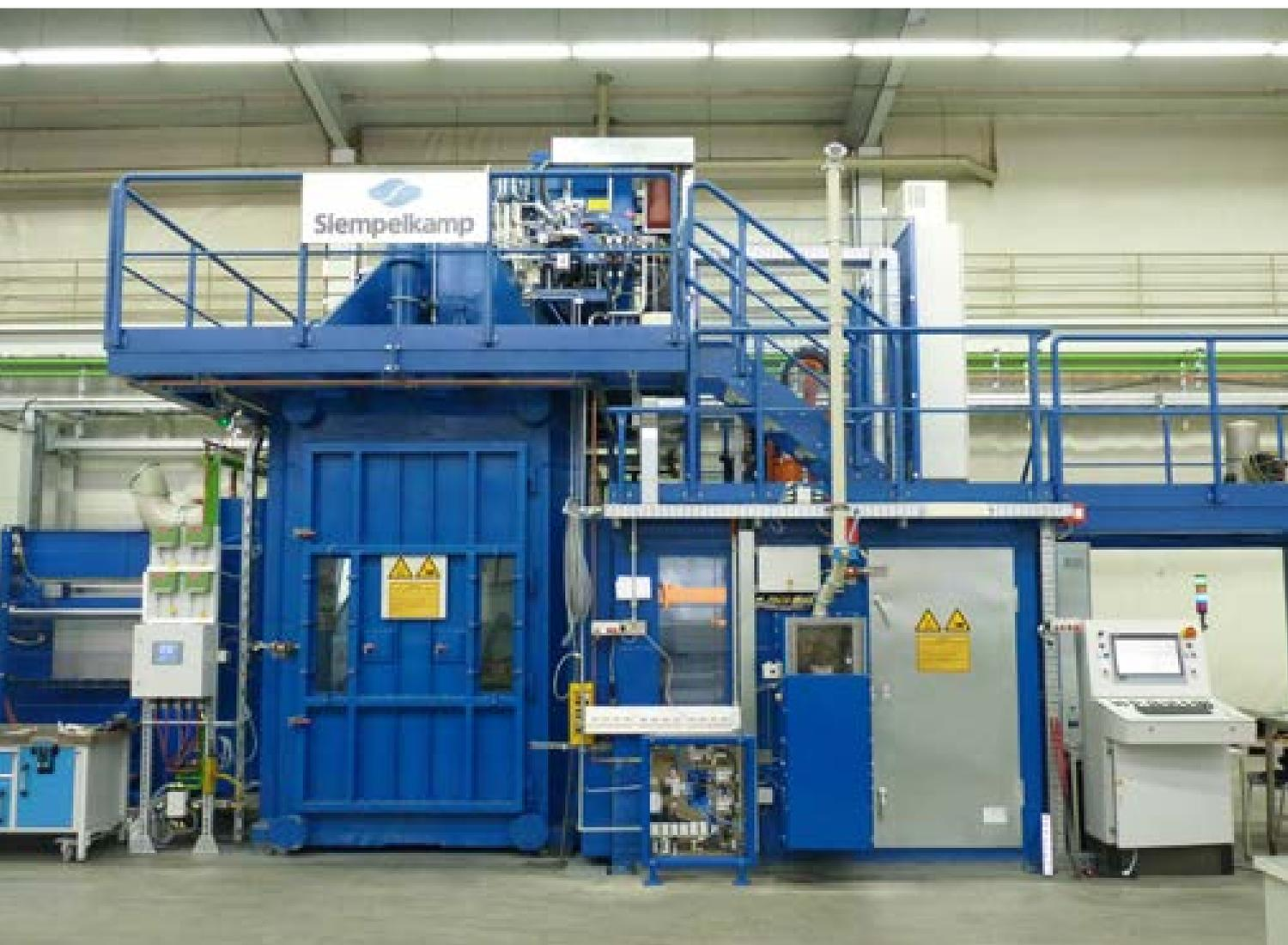
Isothermal forging press, front view
