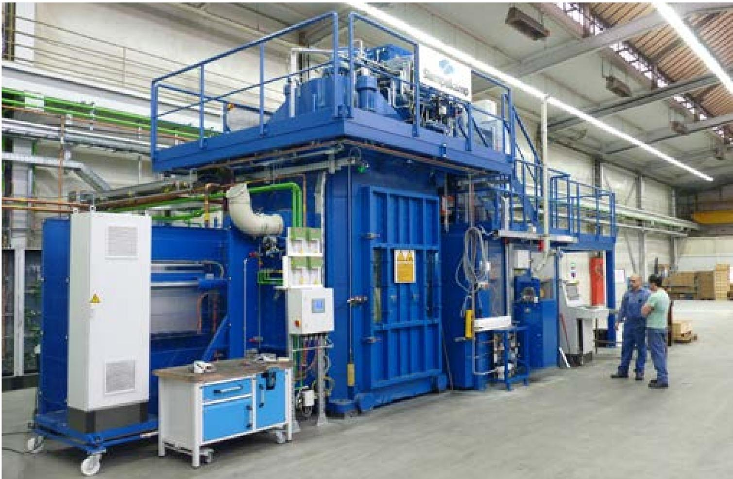
First of three isothermal forging cells for Leistriz
