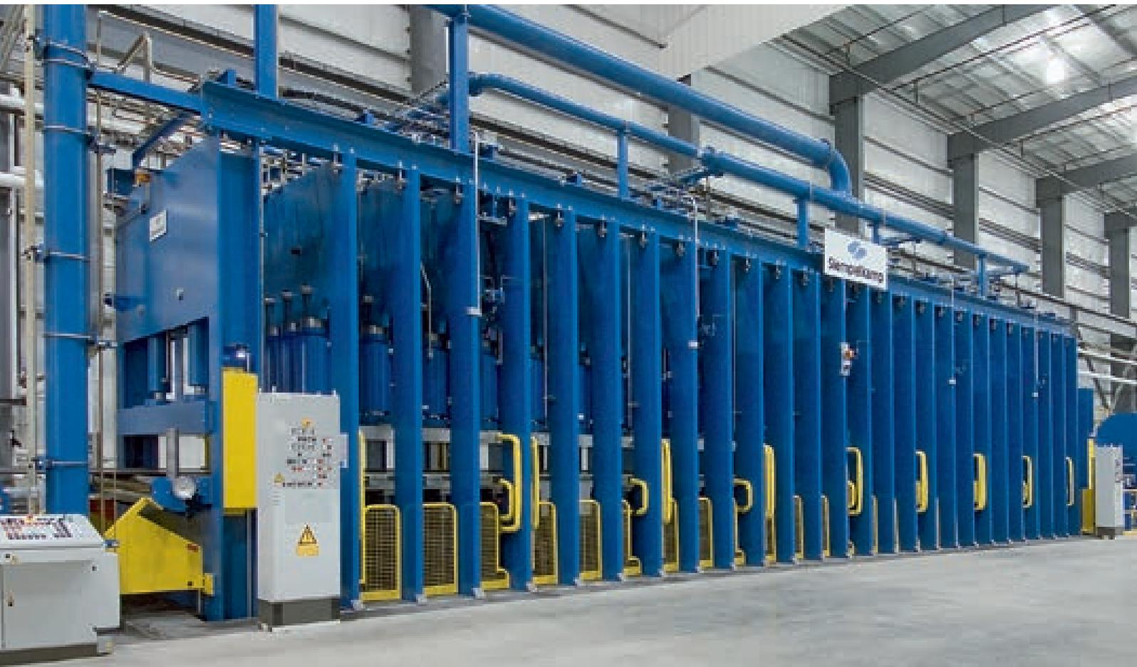
Siempelkamp presses and plants for the rubber industry are characterized by their long life cycles, high efficiency, and transparent process control. They are used for the production of flooring materials, rubber sheets and mats with smooth surfaces as well as conveyor belts.
