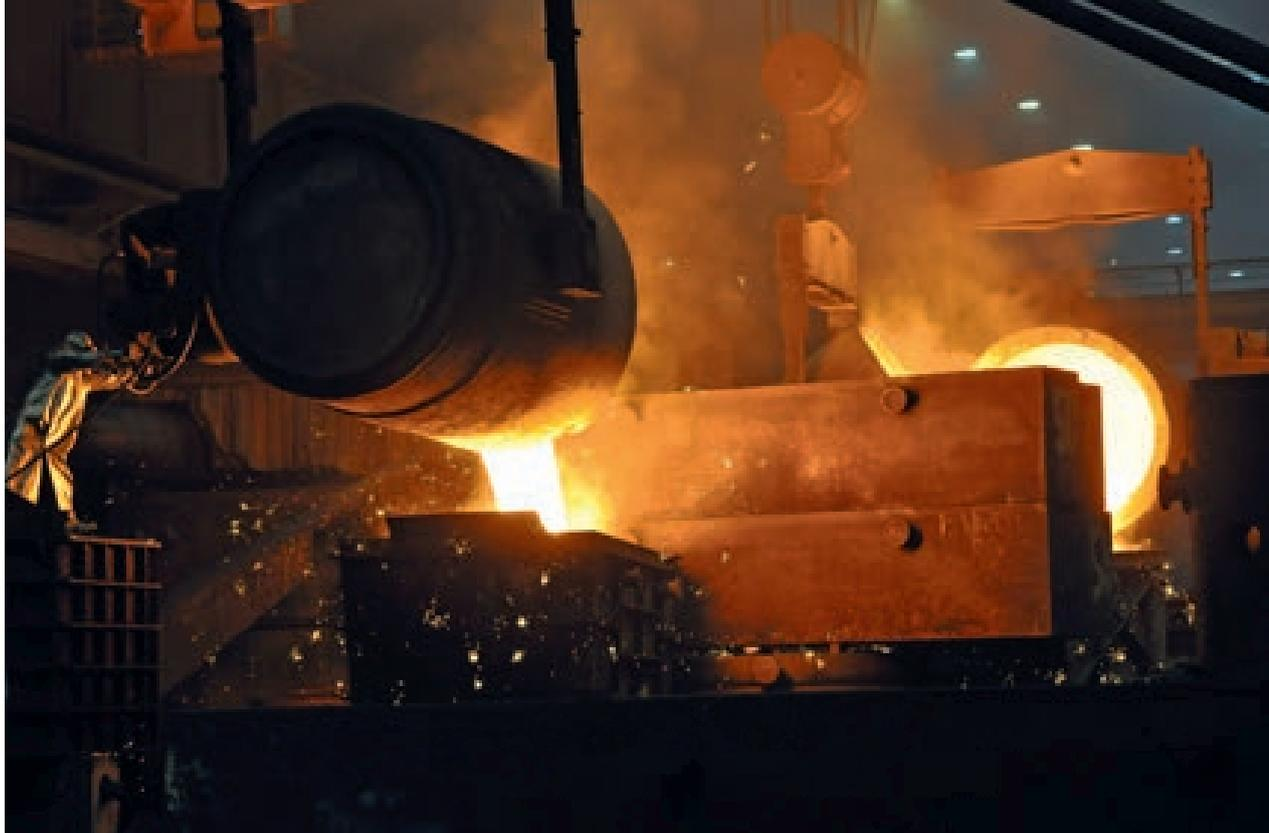
Casting of a CASTOR® cask body with a melting temperature of 1,320 °C
