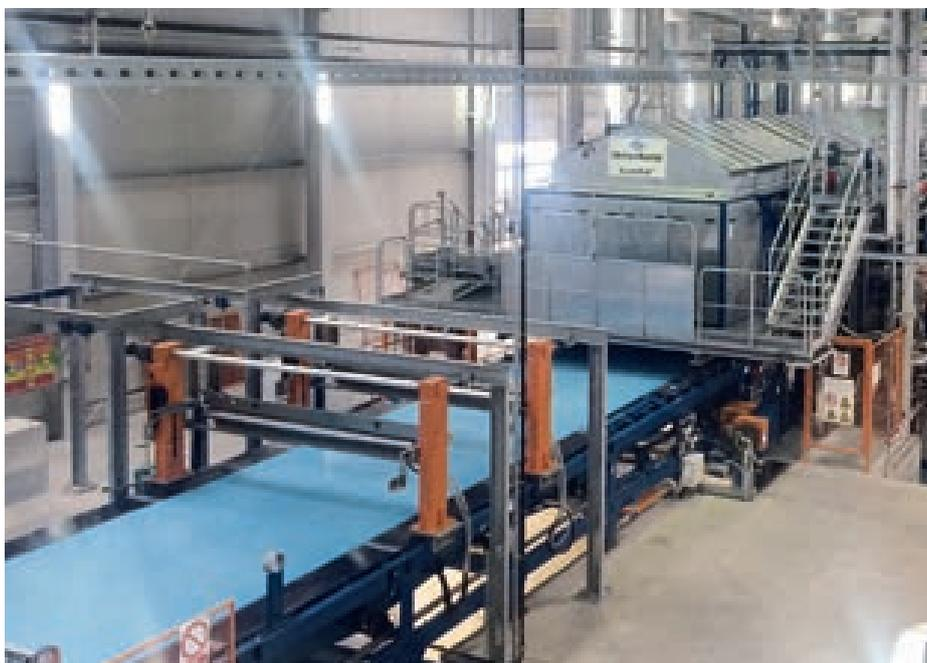
From left to right: the pre-press with trimming saw and press infeed
