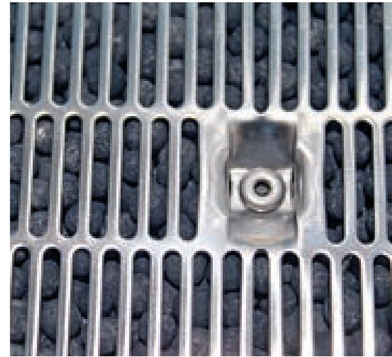
Catalyst material filled into a cartridge
