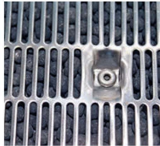
Catalyst material filled into a cartridge
