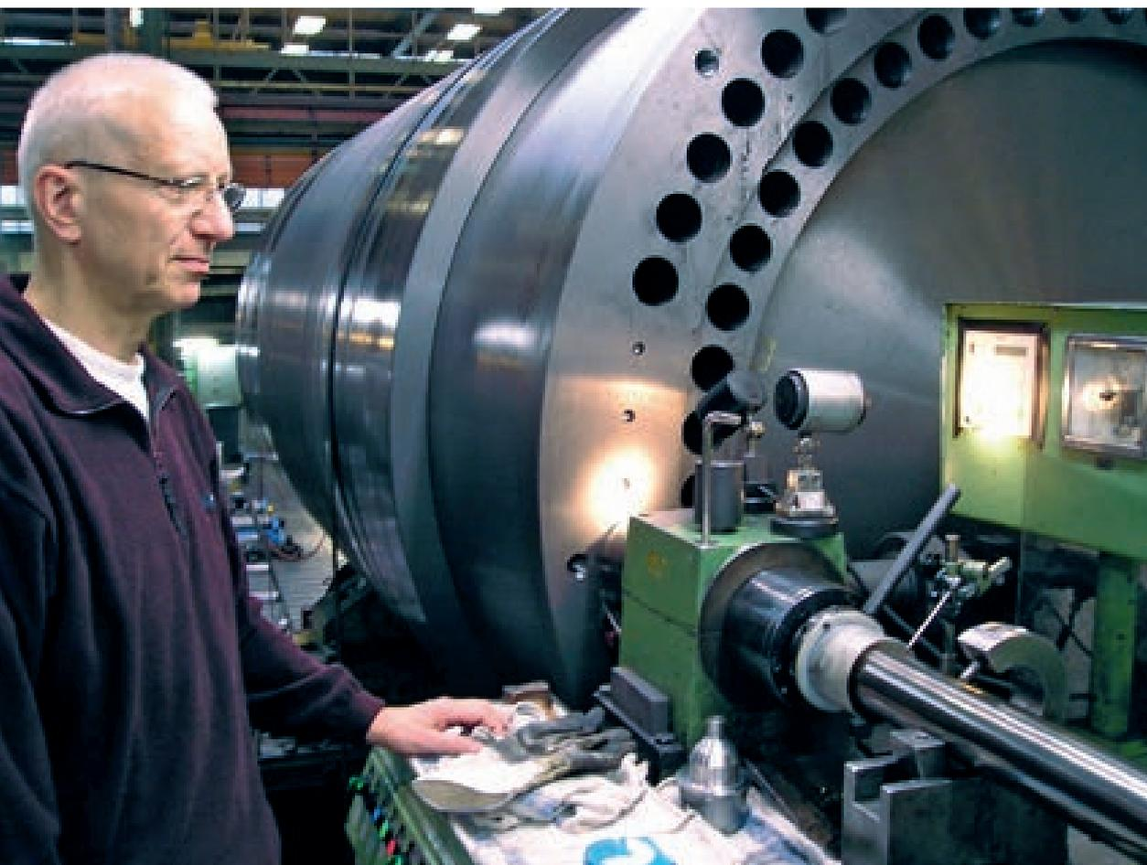
Deep hole drilling on a CASTOR® cask body
