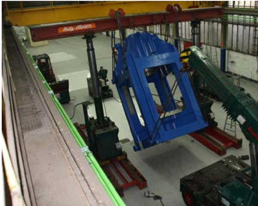
Insertion of the one-piece press body consisting of nodular graphite cast iron
