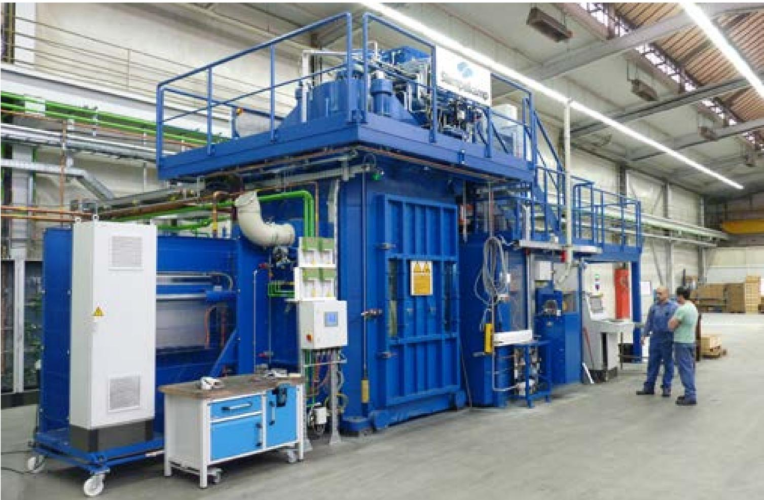
First of three isothermal forging cells for Leistriz
