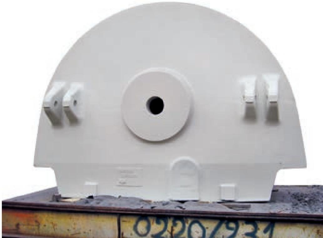
Cast component for a tile press
